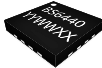
3mm x 3mm x 0.75mm, 16-Lead TQFN Package
